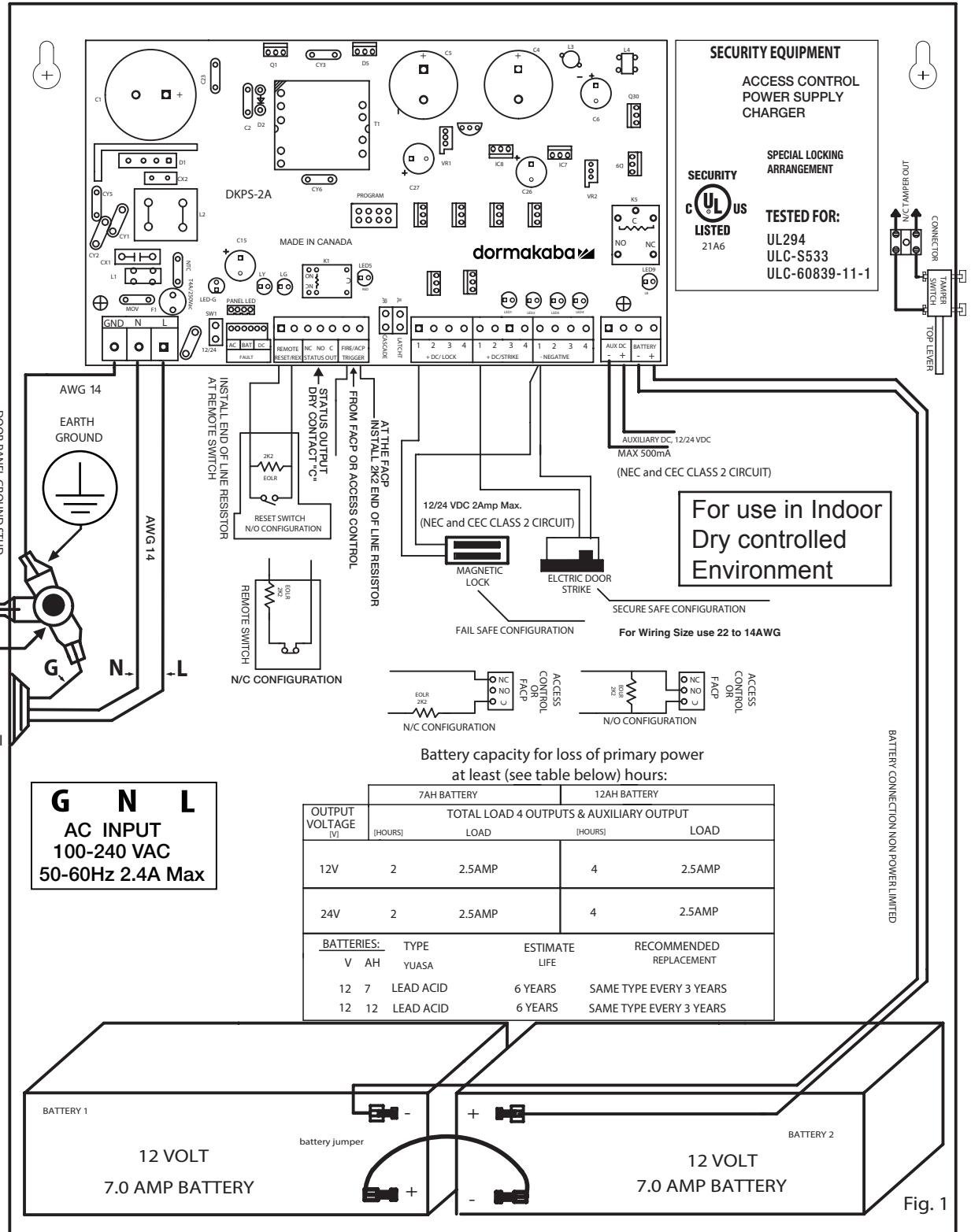
KEEP POWER LIMITED WIRING FROM NON POWER LIMITED WIRING AT LEAST 0.25" INCH APART
