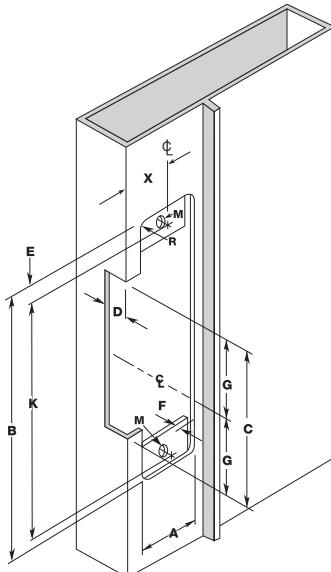
5. Attach the strike insert (coil unit or "motor") to the lip bracket with the small machine screws provided. (M4 x 9.5mm)
