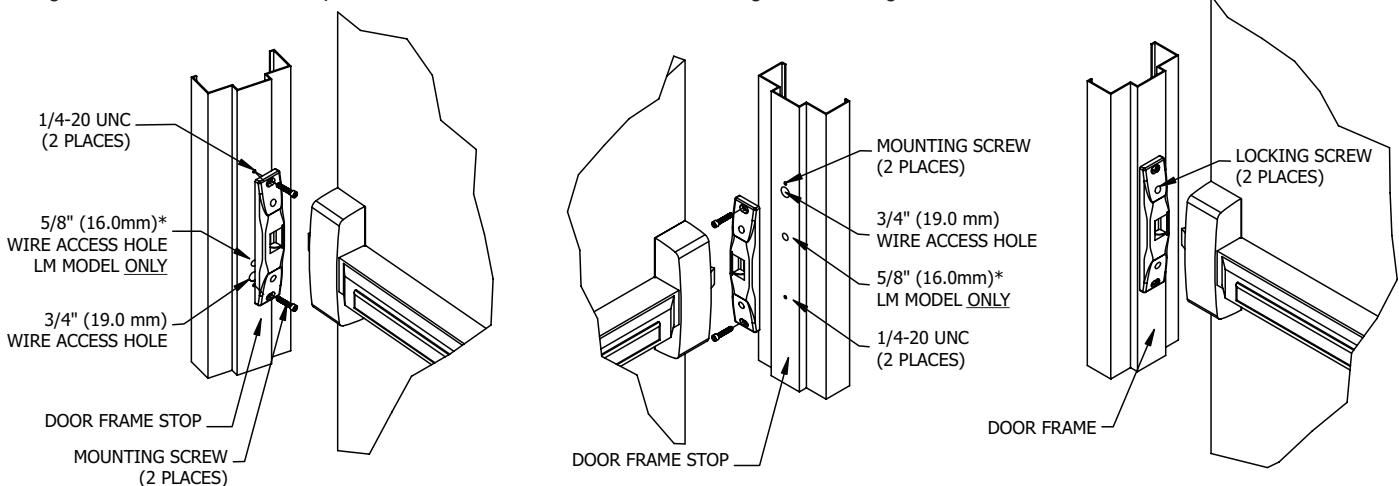
**NOTE:** Wire access hole locations are relative to the exit device orientation. **NOTE:** \*Second wire access hole required for monitor wires
