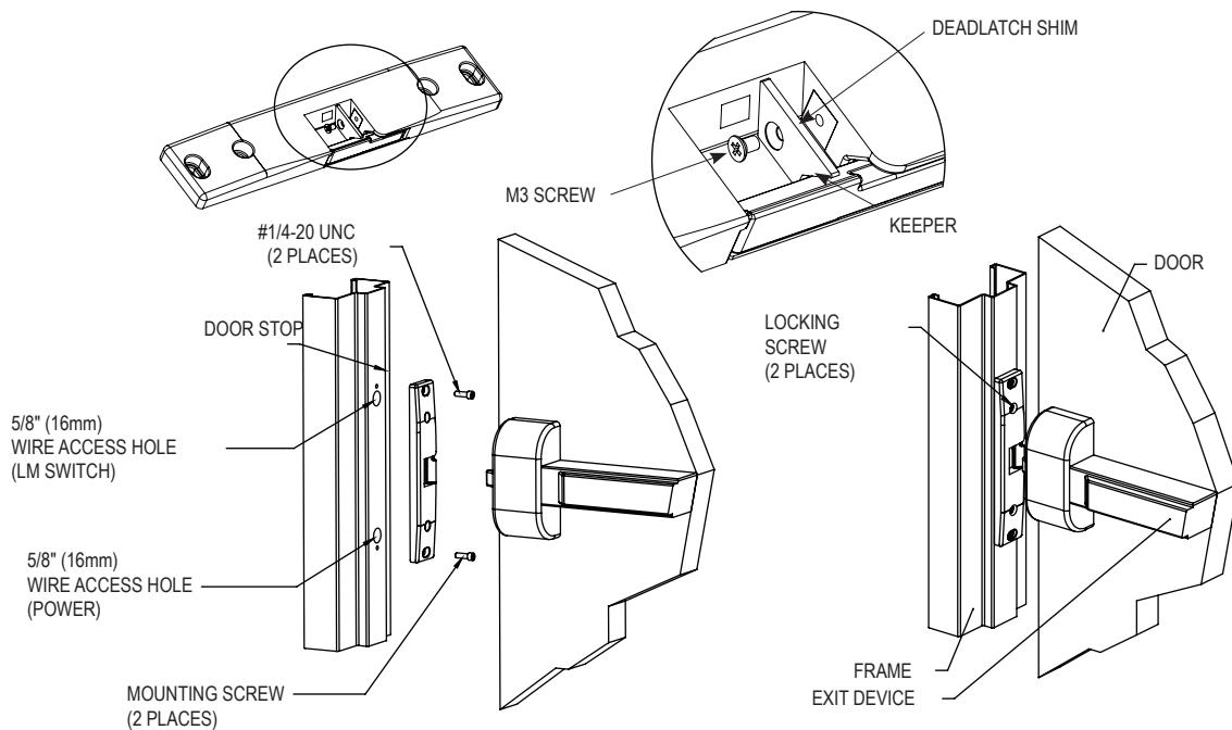
**NOTE:** Wire access hole locations are relative to the exit device orientation.
