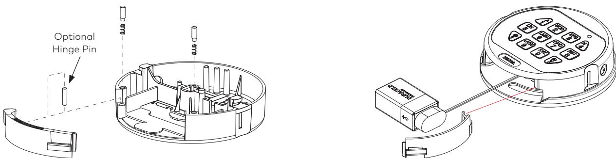
Without the hinge pin the battery door is detached during opening. To reinstall it, orient the hinge hook to the right, place the hinge hook onto the battery door post of the keypad, and rotate clockwise to the left until the handle is secured inside the left edge of the keypad housing.
